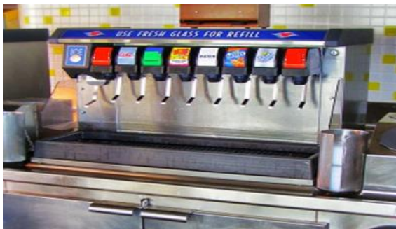
Equipment Sealed to Counter Top
