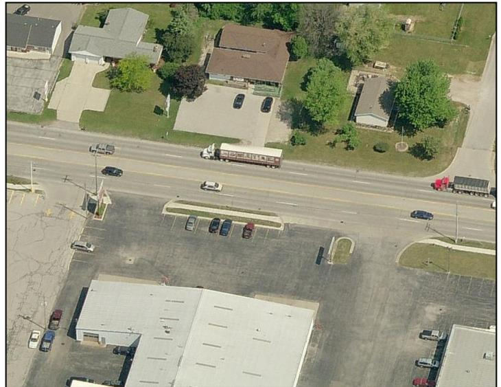
Δ ***Substandard driveway design/storage;*** small driveway radii, too little driveway storage (distance from roadway to first internal parking/circulation) at numerous locations - typically at the older small commercial sites.
